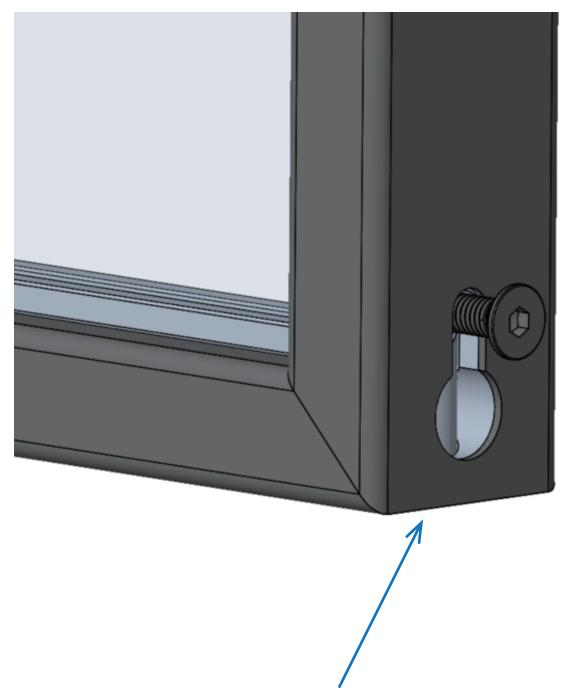
For the bottom one, drill one hole on the floor and insert the pin to the floor then fix it with the bolt
